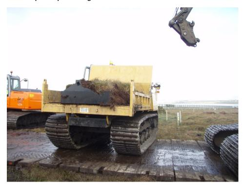
2d. Lift bucket + turve off back of truck and place on turve storage area
